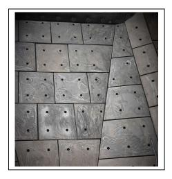
Full-face-liners with casted in bolts for fastening. The design is ideal for applications with an impact angle of 45-135 degrees from the surface.
