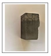
The picture to the left shows a piece Inomet material after destructive analysis. The metallurgical bond between tungsten carbide and ductile cast iron gives a composite material with high quality adhesion to the tungsten carbide.
